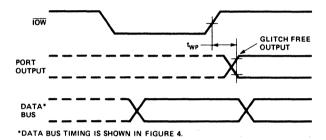
Figure 3. I/O Port Timing
